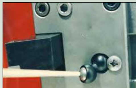
BugEye shown installed on CNC turning center.
